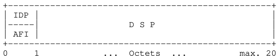
Figure 5 Structure of NSAP Addresses (AFI=0x50 or AFI=0x48)
