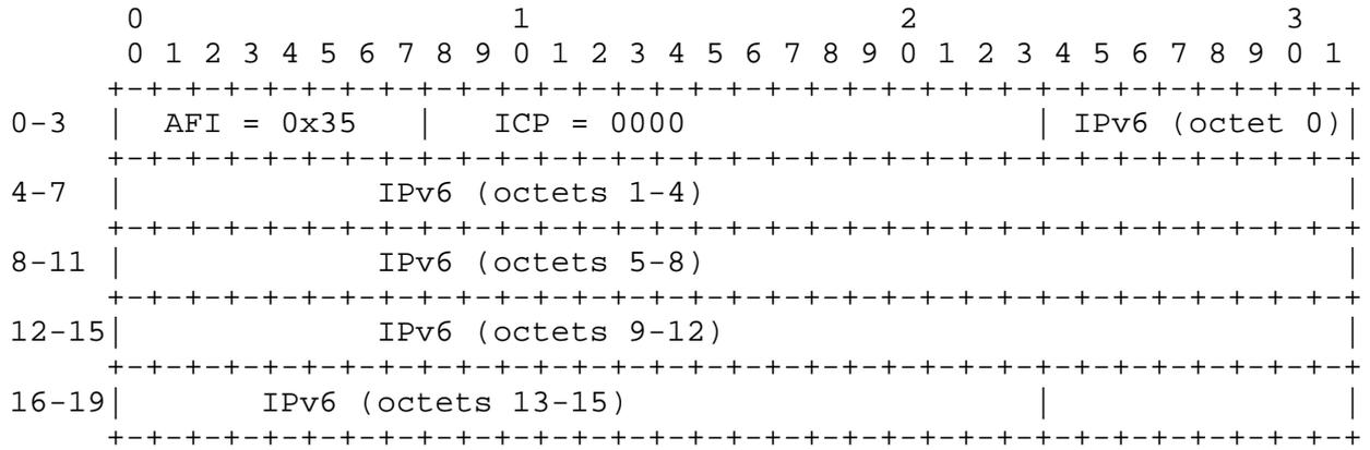
An NSAPA with the IANA AFI code and ICP set to '0' (zero) is converted to an IPv6 address by stripping off the first 3 octets and the 20th octet. If the NSAP-addressed contents are passed to a higher layer, the last octet SHOULD be presented to the higher layer as well.
