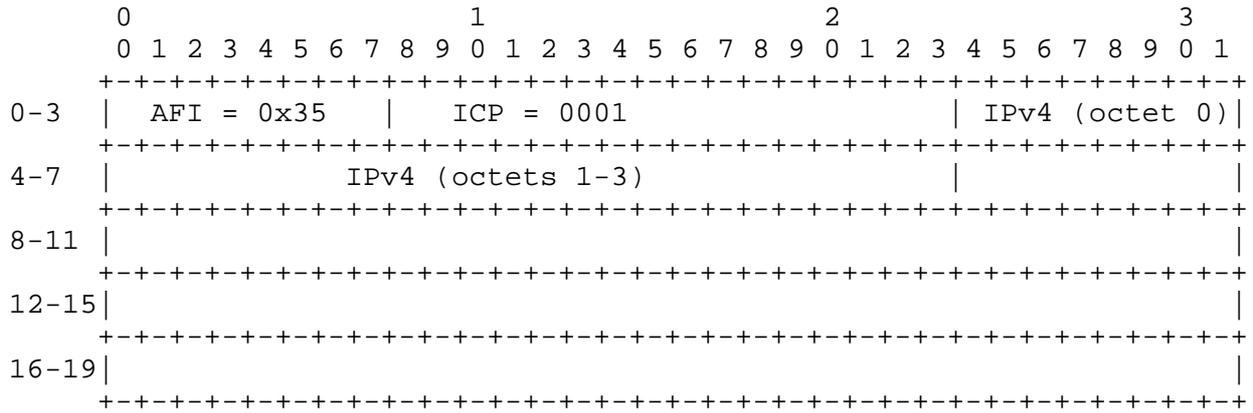
An NSAPA with the IANA AFI code and ICP set to '1' (one) is converted to an IPv4 address by stripping off the first 3 and the last 13 octets. If the NSAP-addressed contents are passed to a higher layer, the last 13 octets SHOULD be presented to the higher layer as well.
