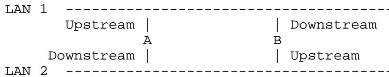
B will unconditionally forward packets from LAN 1 to LAN 2, and A will unconditionally forward packets from LAN 2 to LAN 1. This will cause an upstream loop. A multicast routing protocol that employs a tree building algorithm is required to resolve loops like this.
