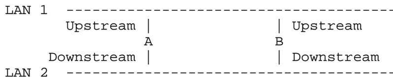
LAN 2 can have two proxy devices, A and B. In such a configuration, one proxy device must be elected to forward the packets. This document requires that the forwarder must be the IGMP/MLD querier. So proxy device A will forward packets to LAN 2 only if A is the querier. In the above figure, if A is the only proxy device, A can be configured to forward packets even though B is the querier.
