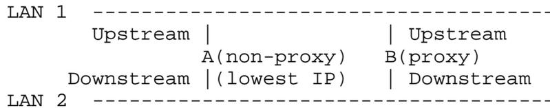
Device A has the lowest IP address on LAN 2, but it is not a proxy device. According to IGMP/MLD Querier election rule, A will win the election on LAN 2 since it has the lowest IP address. Device B will not forward traffic to LAN 2 since it is not the querier on LAN 2.
