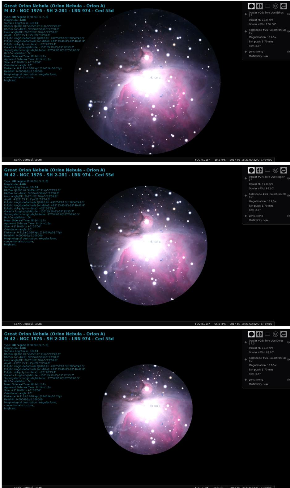
Figure 15.17: Comparing apparent fields of view of (top) a 17 mm Tele Vue Ethos eyepiece with an aFOV of 100°. Magnification is 119.5×. (center) a 17 mm Tele Vue Nagler eyepiece with an aFOV of 82°. Magnification is 119.5×. (bottom) a 17.3 mm Tele Vue Delos eyepiece with an aFOV of 62°. Magnification is 117.5×.
