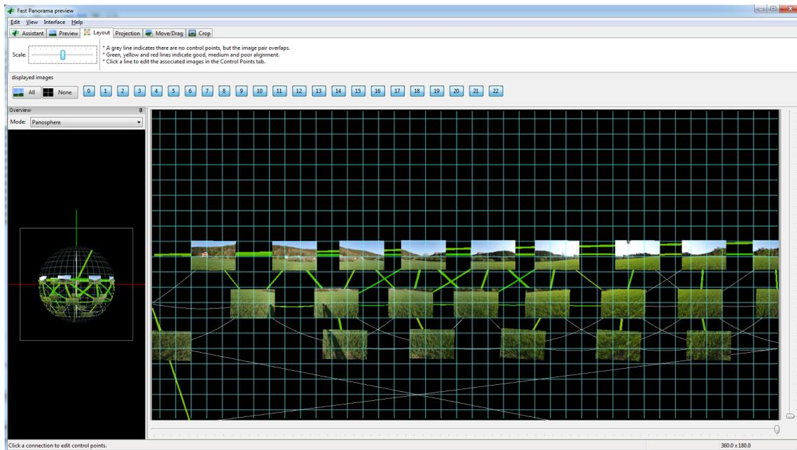
Figure 7.6: **Hugin's** Fast Panorama Preview can be used to check which images are connected to its neighbours. Most important are good matches along the horizon, the images in the lower rows are clearly less important. If captured on a tripod, they should still match.
