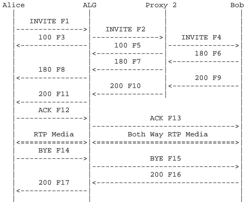
Alice completes a call to Bob through a ALG (Application Layer Gateway) and a SIP Proxy. The routing through the ALG is accomplished using a pre-loaded Route header in the INVITE F1. Note that the media stream setup is not end-to-end - the ALG terminates both media streams and bridges them. This is done by the ALG modifying the SDP in the INVITE (F1) and 200 OK (F10) messages, and possibly any 18x or ACK messages containing SDP.
