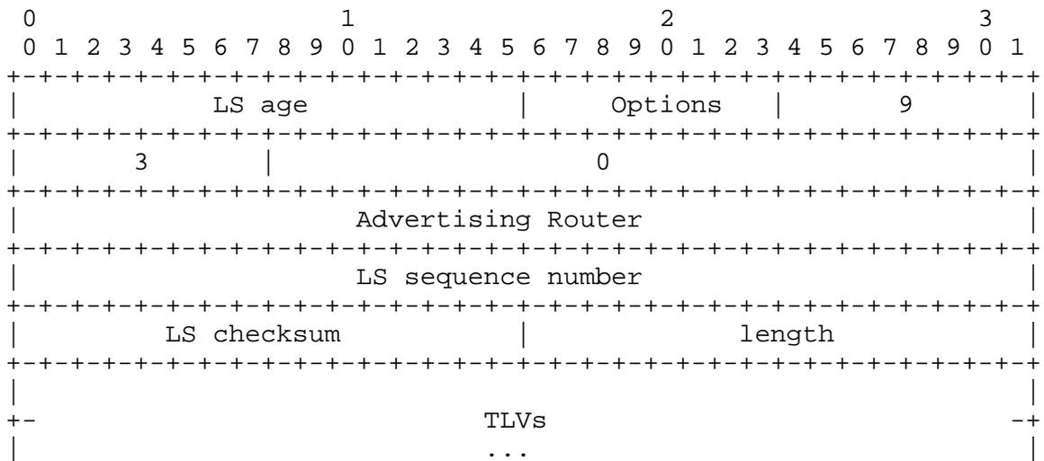
The format of the TLVs within the body of a grace-LSA is the same as the format used by the Traffic Engineering Extensions to OSPF [4]. The LSA payload consists of one or more nested Type/Length/Value (TLV) triplets. The format of each TLV is:
