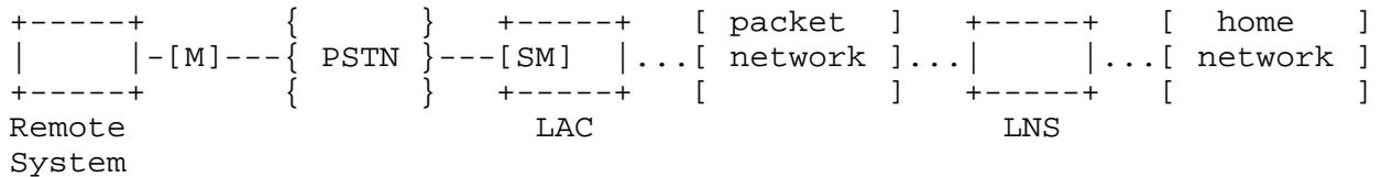
If the LAC implements the functionality described here, it can signal to the LNS when the client modem has gone on-hold and when it comes back online.
