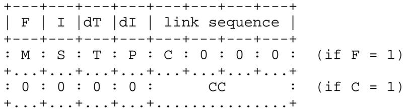
The bits marked "0" in the second flag byte and the CC byte SHOULD be set to zero by the sender and SHOULD be ignored by the receiver.
