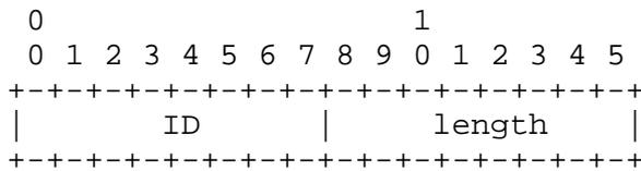
The 8-bit ID is the local identifier of this element in the range 1-255 inclusive. In the signaling section, the range 1-256 is referred to as the valid range, with the values 1-255 referring to extension elements, and the value 256 referring to the 4-bit field 'appbits' (above).
