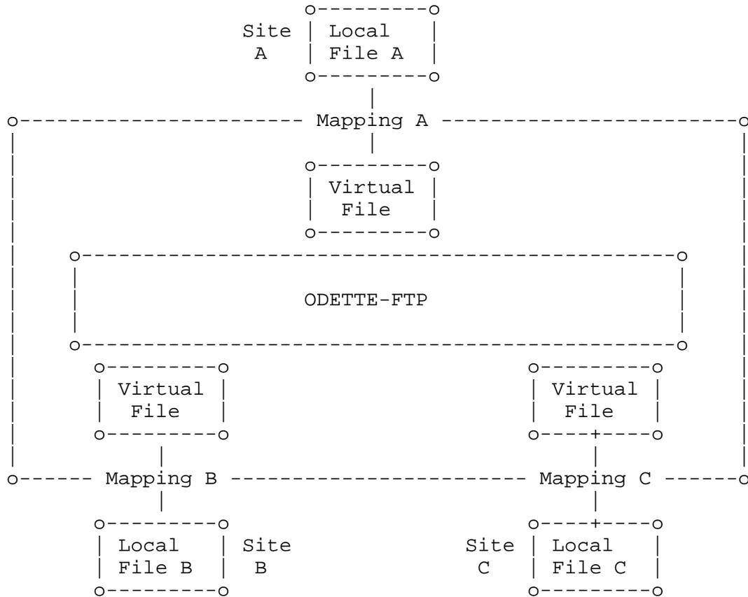
A Virtual File is described by a set of attributes identifying and defining the data to be transferred. The main attributes are detailed in Sections 1.5.1 to 1.5.4.
