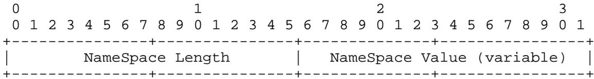
It is important to note that the priority (i.e., "r-priority" token syntax) from [rfc4412] is NOT used in the ResourcePriority attribute. This is because the objective of the attribute is to advertise the NameSpace associated with a gateway and not the individual priorities within that NameSpace.
